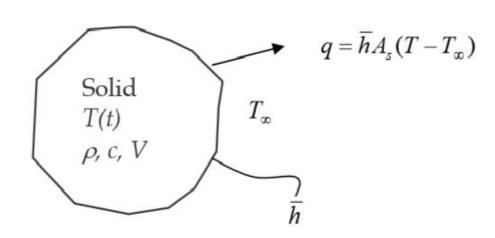
The solid object shown in figure is a metal piece which is being cooled in air after hot forming.
