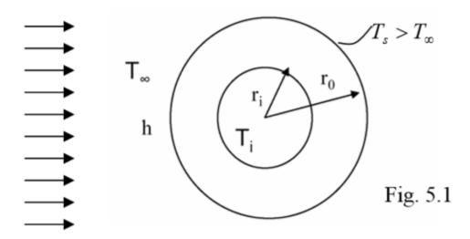
For very large r<sub>i</sub>, the heat transfer rate by conduction through the cylinder wall is approximately
